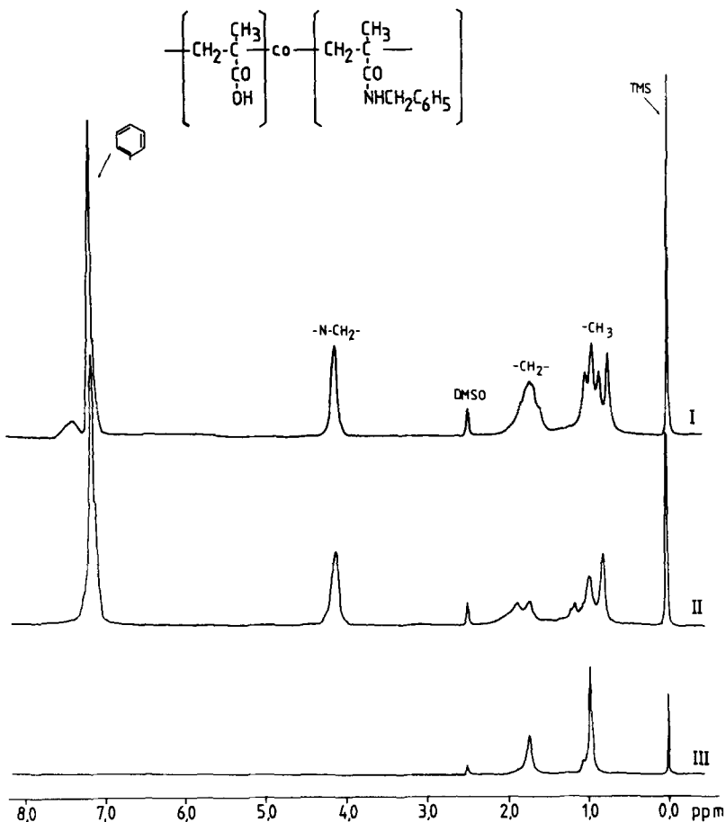
Fig. 1 1 H-NMR spectra of a syndiotactic methacrylic acid-methacryloyl-N-benzyl amide copolymer (trace I), an atactic poly(methacryloyl-N-benzyl amide) (trace II), and syndiotactic poly(methacrylic acid) (trace III)
